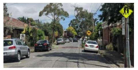
The footpaths along Nelson Street do not meet community access standards. That are narrow, do not feature nature strips, frequently interrupted by tree plantings, signage and obstacles (motorbikes, bins, etc), and uneven driveways.
